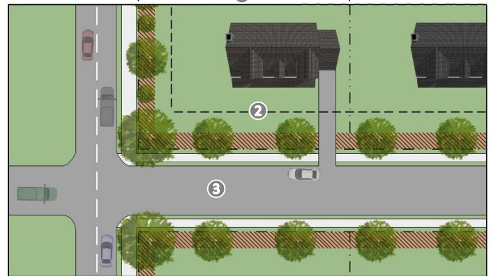
1: RESIDENTIAL PROPERTY; 2: BUILD LINE; 3: COLLECTOR STREET; 4: TEN (10) FOOT LANDSCAPE BUFFER; 5: PERIMETER COLLECTOR OR ARTERIALS ROADWAY
